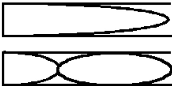
Figure 7(b). First and second pressure modes for a pipe closed at one end.
